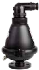
Series 701/75 Combination air valve Orifice sizes: Automatic: 12 mm 2 Kinetic: 804 mm 2 Reinforced nylon Inlet flange or 2"/3" BSP thread PN 10 DN50-100
